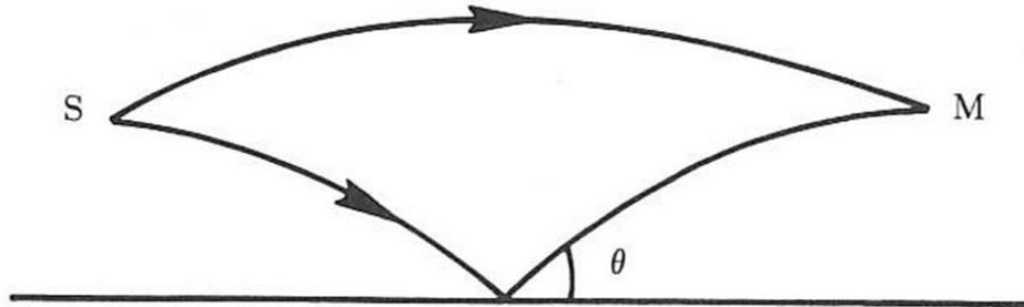
**Figure 1: Depiction of Acoustic Ray Curvature Due to the Ground Proximity Speed Differential from Source, S to Receiver Microphone, M**
