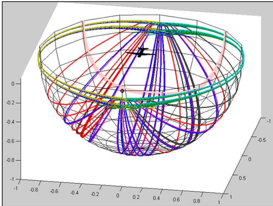
Figure 5: Noise Emission Angles at 1000 ft and 2000 ft AGL
