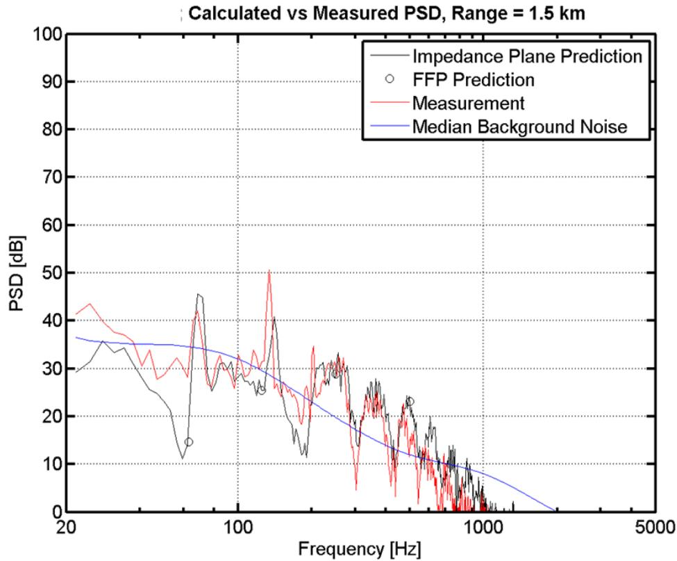
**Figure 7: Measured vs Predicted Spectra of the NRC Convair; Altitude 12000 ft AGL, Range 1.5 km**
