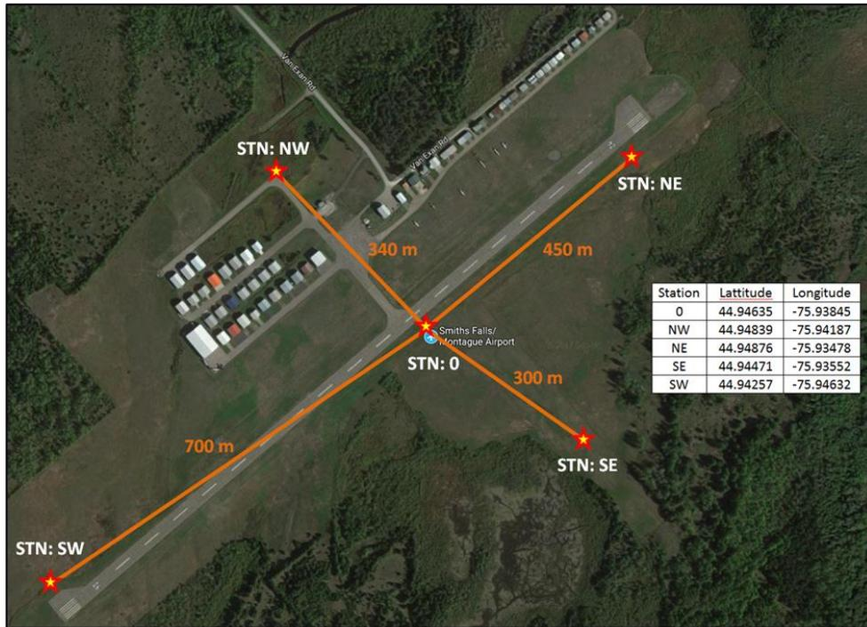
Figure 2: Smiths Falls Montague Airport Acoustic Measurement Locations
