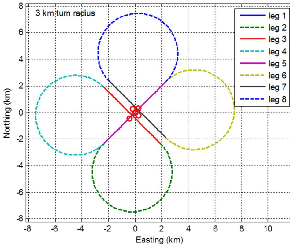
**Figure 4: Overhead Flight Path of the NRC Convair 580 for AGL Flight Altitudes of 1000 ft, 2000 ft, 8000 ft and 12 000 ft**
