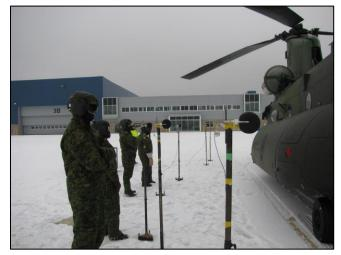
Figure 2: Exterior Noise Measurement
