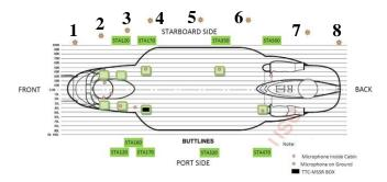
Figure 1: CH-147F Measurement Locations [3]
