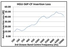
Figure 4: HGU-56P-CF Insertion Loss [5]
