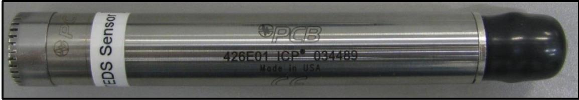
Figure 14: PCB 378B02 ½ inch ICP free-field microphone
