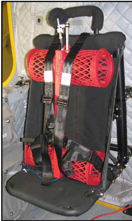
Figure 13: Phase 2 microphone stand strapped into a seat
