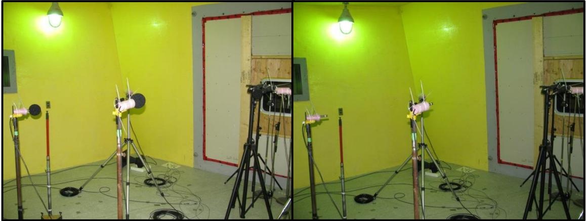
Figure 38: Windscreen insertion loss test setup (Left: Run 1/2, Right: Run 3/4)
