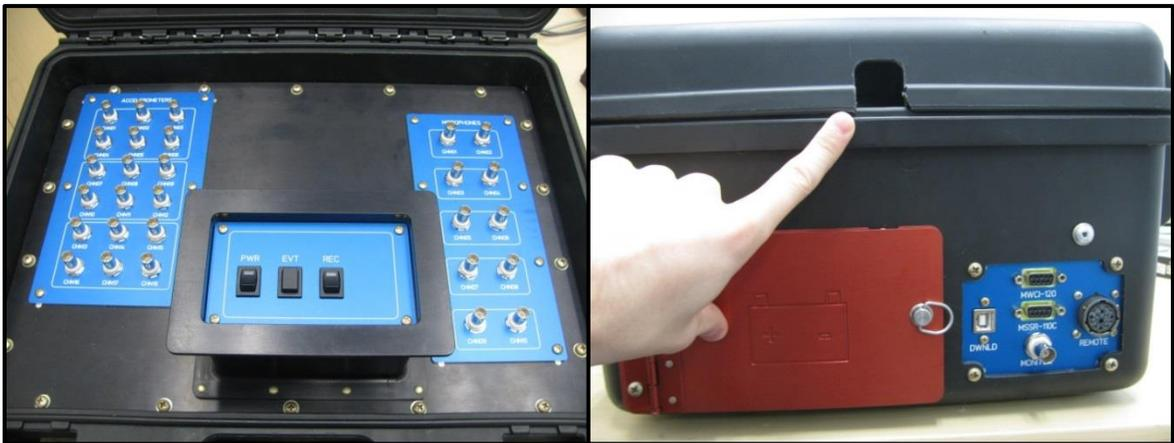
Figure 9: Phase II enclosure box BNC sensor ports and wire exit port
